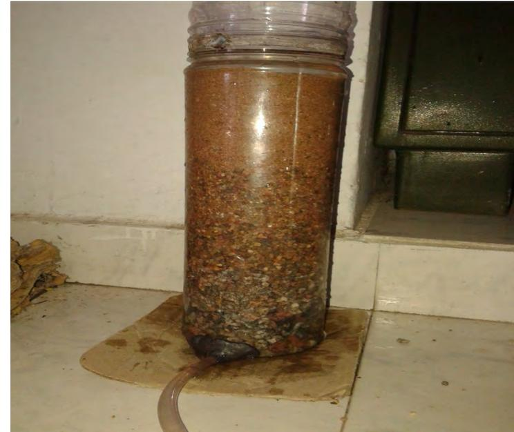
A biosand water filter developed at IIT Kanpur to help purify water
