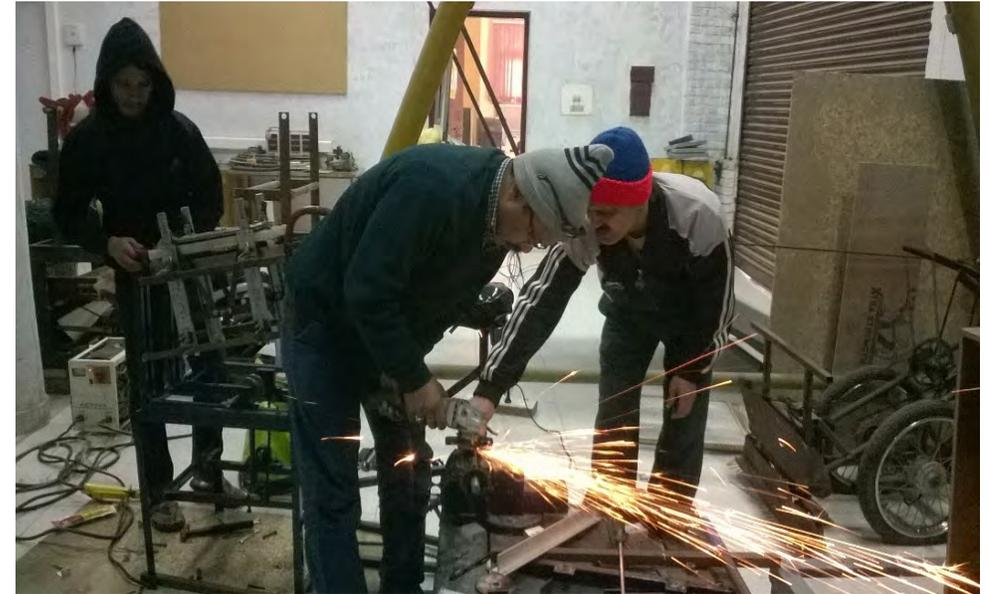
Frame or product platform fabrication using square tube trusses
