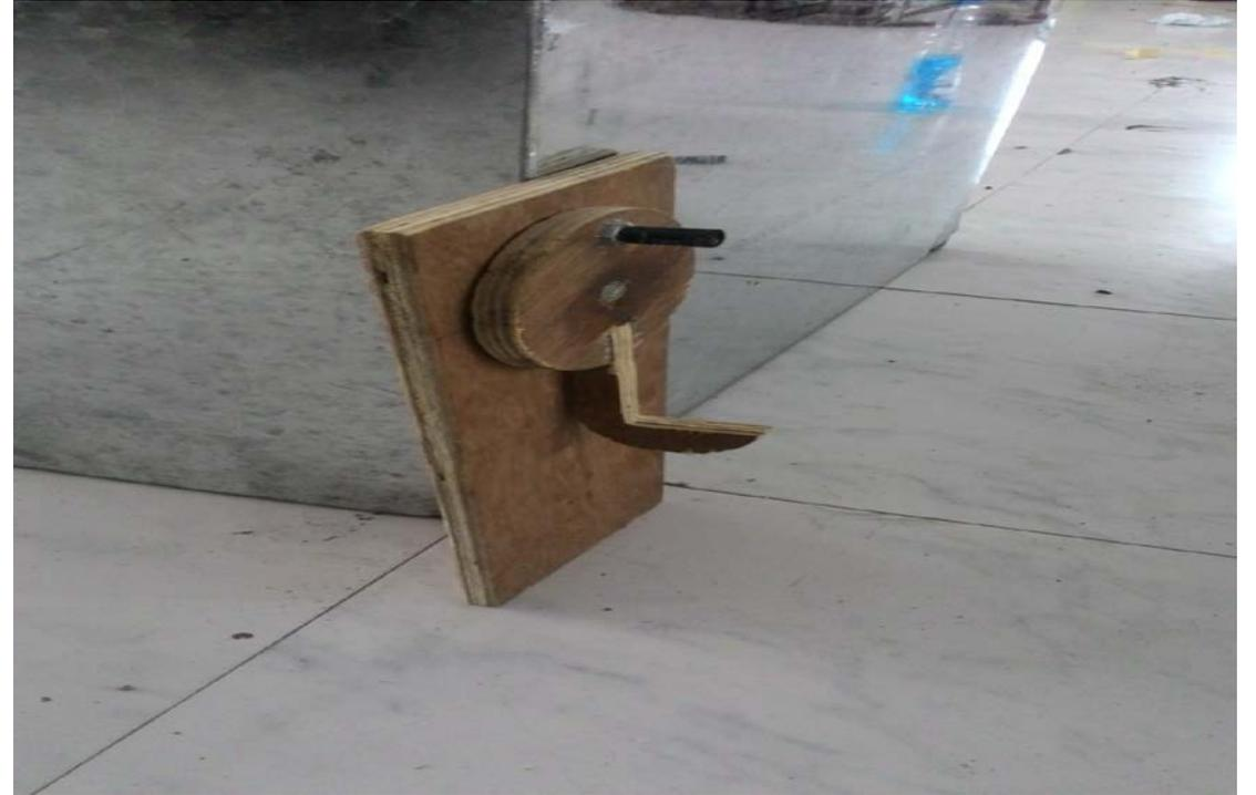
Prototyping using cheap materials such as wood (Crank for De-seeding)
