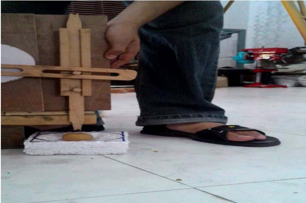
Prototyping of punch created using card-board and plywood
