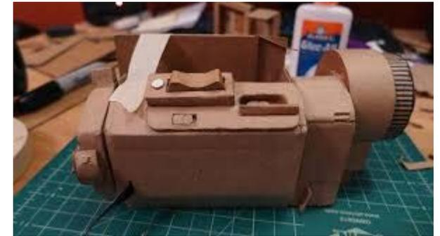
A prototype of printer built from cardboard for testing the variable : Ergonomics of operation
