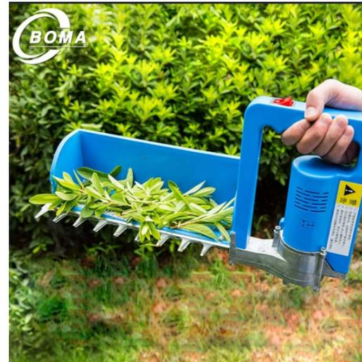
Tea plucking with a motor powered device
