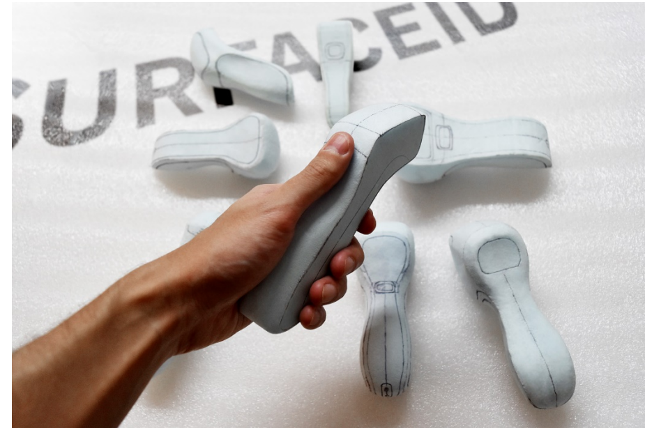
Multiple prototypes of handle to test gripping experience (material is Styrofoam)
