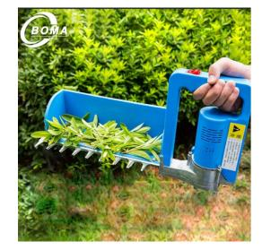
Tea plucking with a motor powered device
