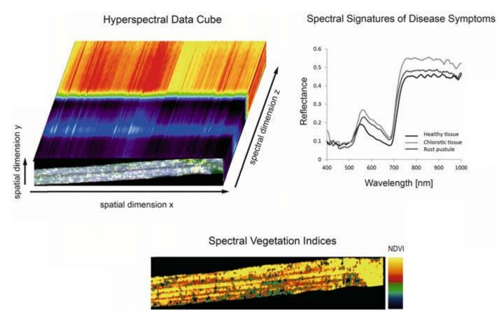
Hyperspectral imaging of barley leaf diseased with brown rust. Each pixel of the 3-dimensional data cube contains a continuous spectral signature from 400 to 1,000 nm. Based on this imaging data spectral vegetation indices maps may be calculated
